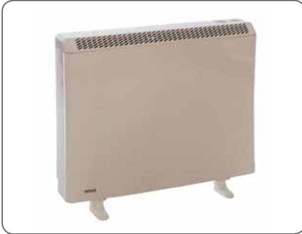
These heaters use cheaper off-peak (Economy 7) electricity during the night. They store the heat, which is then given out when it is needed during the day. They have two controls, one called Input (may be called “Auto-set control”, or “Charge”), the other called Output (“Room temperature”, or “Boost”).
